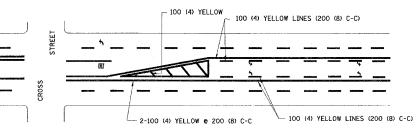
A MINIMUM OF TWO PAIRS OF TURN ARROWS SHALL BE USED, WHITE IN COLOR. ADDITIONAL PAIRS SHALL BE PLACED AT 60 m (200') TO 90 m (300') INTERVALS.
