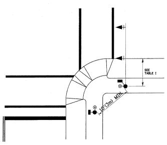
RECOMMENDED PUSHBUTTON LOCATIONS FOR ACCESSIBLE PEDESTRIAN SIGNALS SHALL BE IN ACCORDANCE WITH THE CURRENT MUTCO (SEE NOTE 1). TO MEET MUTCO REQUIREMENTS, PEDESTRIAN SIGNAL PUSHBUTTONS MAY HAVE TO BE MOUNTED ON A SEPARATE POST.
