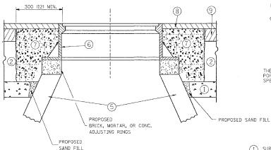
EXISTING BROKEN FRAMES AND LIDS SHALL BE REMOVED AND DISPOSED OF BY THE CONTRACTOR AND SHALL BE REPLACED AS DIRECTED BY THE ENGINER, REPLACEMENT FRAMES AND LIDS WILL BE PAID FOR IN ACCORDANCE WITH ARTICLE 109.04 OF THE STANDARD SPECIFICATIONS UNLESS A SEPARATE PAY ITEM HAS BEEN PROVIDED.
