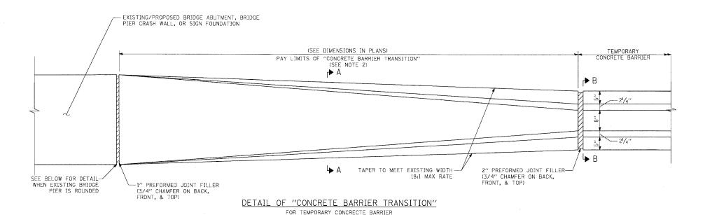
INCLUDED IN THE COST OF CONCRETE BARRIER TRANSITION PAY LIMITS OF "CONCRETE BARRIER TRANSITION" EXISTING/PROPOSED BRIDGE ABUTMENT, BRIDGE — PIER CRASH WALL, OR SIGN FOUNDATION ABOVE DETAIL 1" PREFORMED JOINT FILLER— (3/4" CHAMFER ON BACK, FRONT, & TOP) -45° CHAMEER
