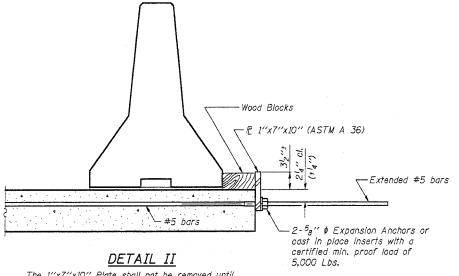
The 1''x7''x10'' Plate shall not be removed until Stage II Construction forms and all reinforcement bars are in place and the concrete is ready to be
