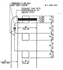
\*\* UNIT DUCT IS TO BE SHOWN ON PLAN SHEETS BUT SHALL NOT BE INCLUDED IN THE PAY ITEMS. NOTE: DUAL LEFT TURNS NOT SHOWN REFER TO PLAN SHEET FOR DETECTOR LOOP REPLACEMENT VOLUME DENSITY ("FAR OUT" DETECTION)
