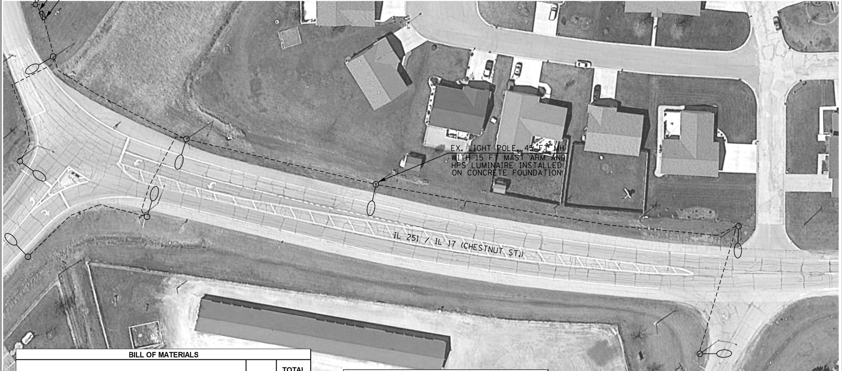
EX. LIGHT POLE, 45 FT MH WITH 15 FT MAST ARM AND HPS LUMINAIRE INSTALLED ON CONCRETE FOUNDATION
