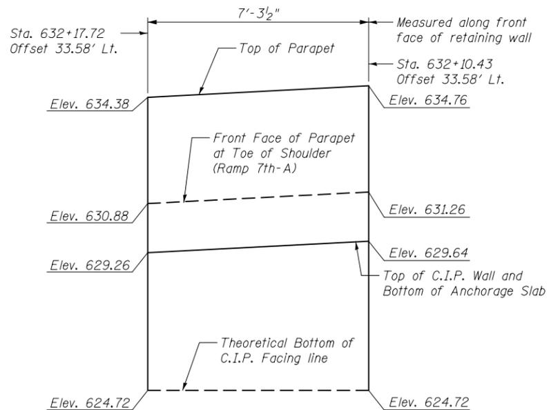
**ELEVATION VIEW OF C.I.P. FACING ALONG RAMP 7th-A**
