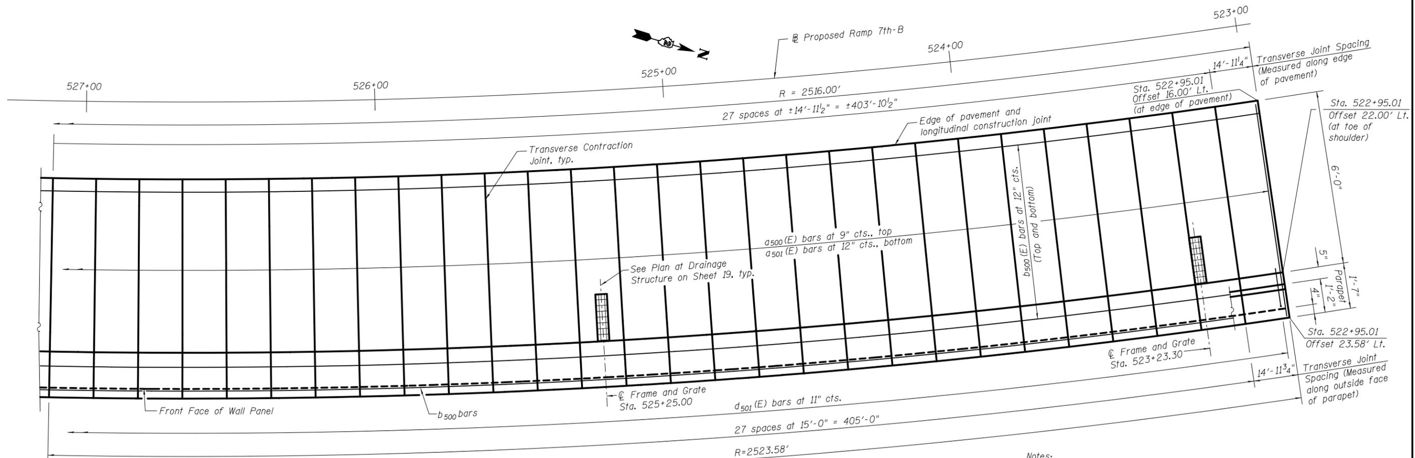
**PARTIAL PLAN - RAMP 7th-B PARAPET AND ANCHORAGE SLAB**
