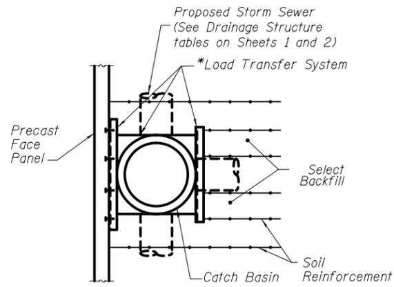
**ANCHORAGE SLAB INLET PLAN**
