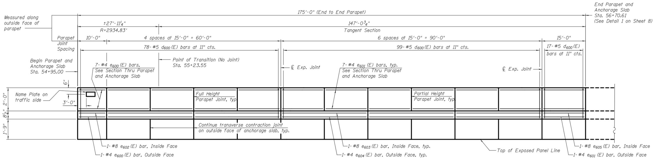
**OUTSIDE ELEVATION OF I-74 EB PARAPET AND ANCHORAGE SLAB**
