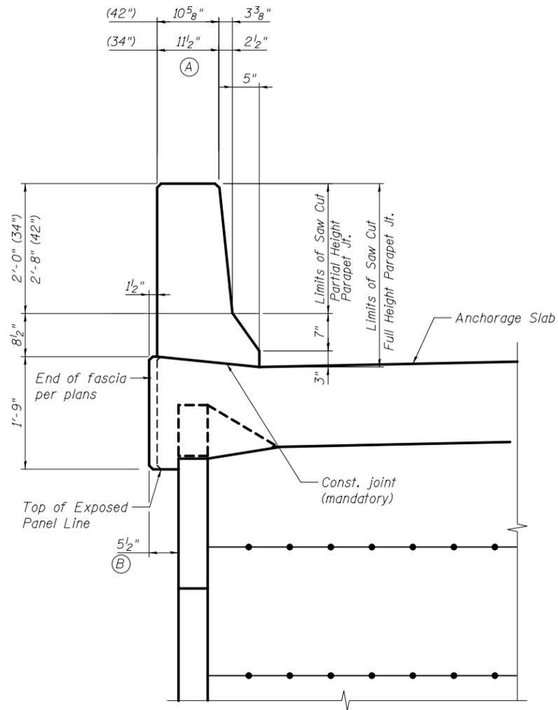
**SECTION THRU PARAPET AND ANCHORAGE SLAB**
