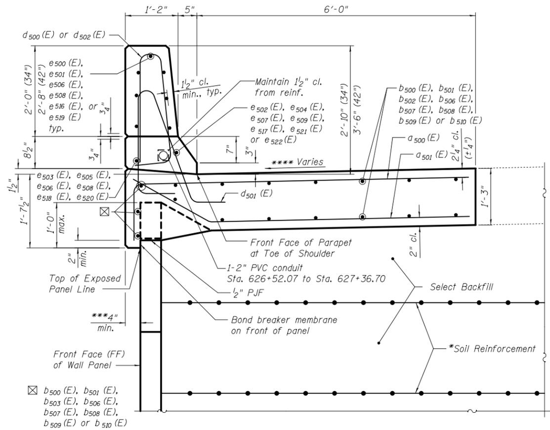
**SECTION THRU PARAPET AND ANCHORAGE SLAB DETAIL**
