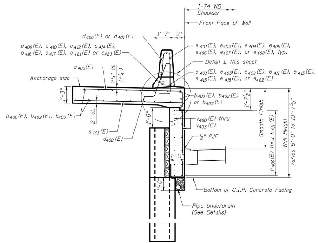
**SECTION THRU PARAPET, ANCHORAGE SLAB AND CONCRETE FACING**
