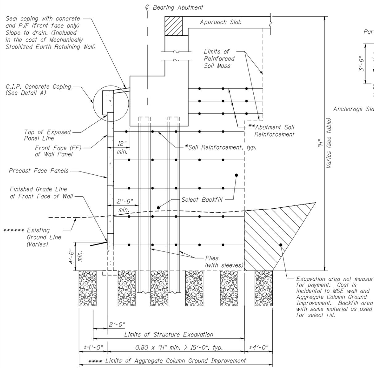
**TYPICAL WALL SECTION THRU ABUTMENT**
