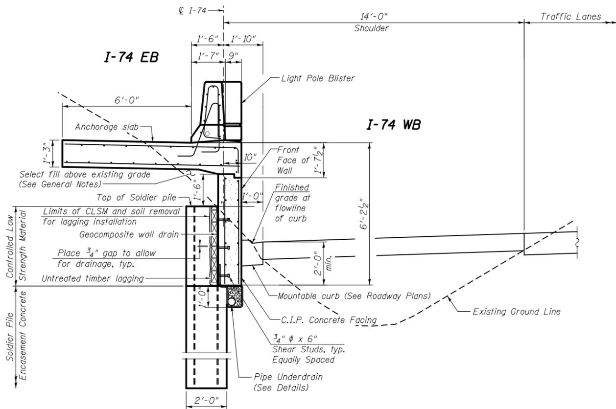
**TYPICAL WALL SECTION AT LIGHT POLE**
