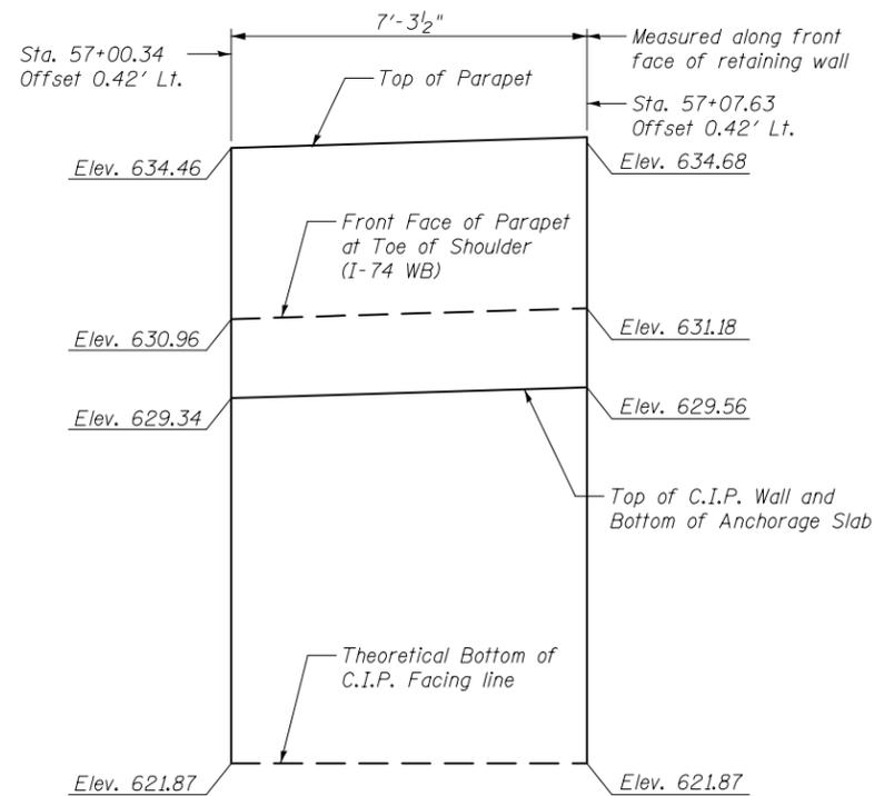
**ELEVATION VIEW OF C.I.P. FACING ALONG I-74 WB**
