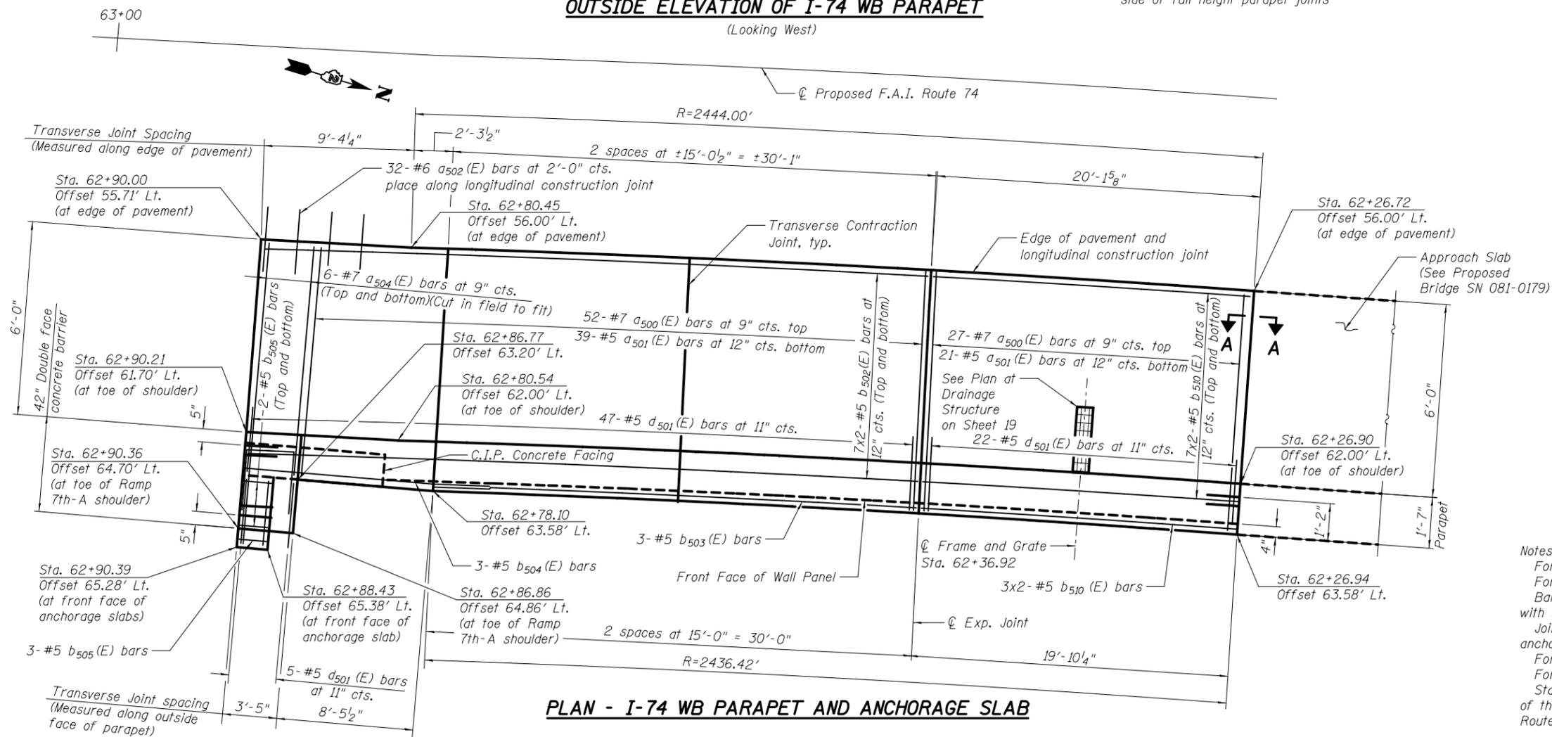
**PLAN - I-74 WB PARAPET AND ANCHORAGE SLAB**
