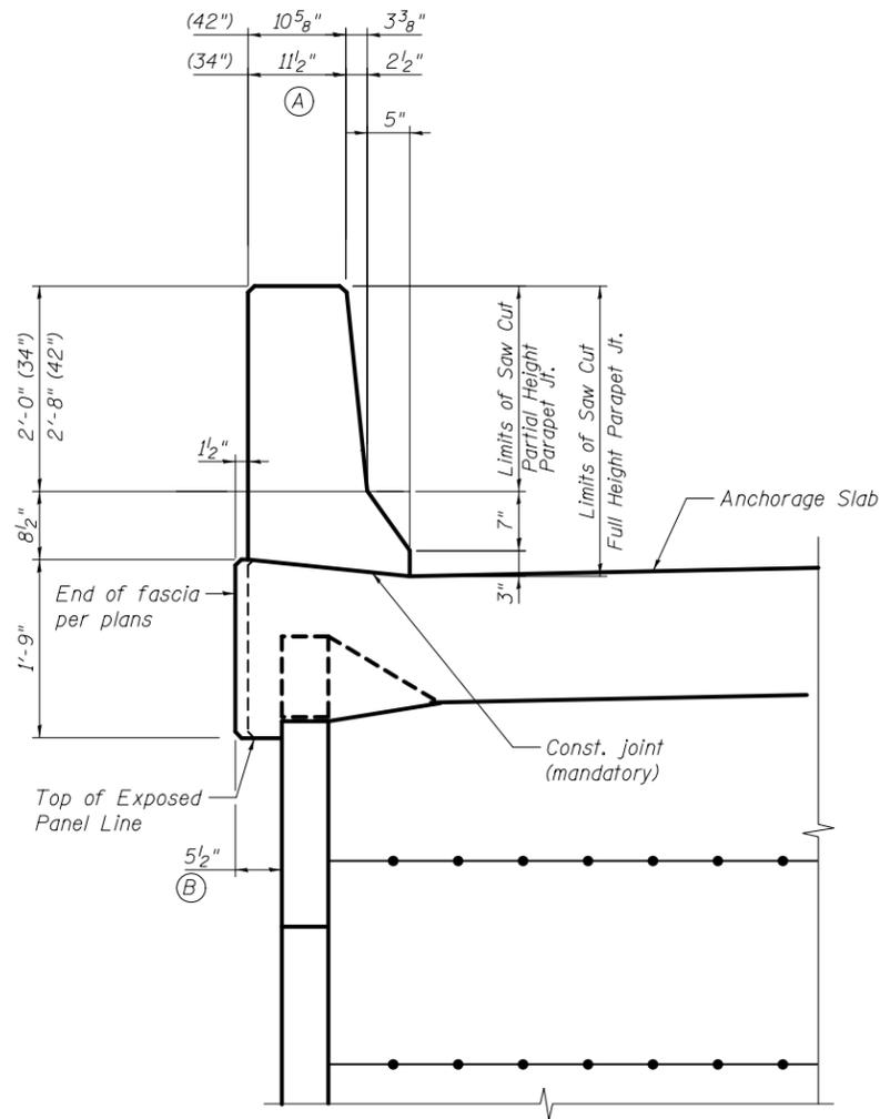
**SECTION THRU PARAPET AND ANCHORAGE SLAB**
