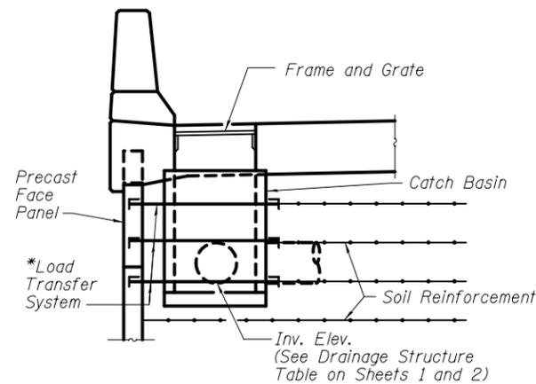
**ANCHORAGE SLAB INLET SECTION**
