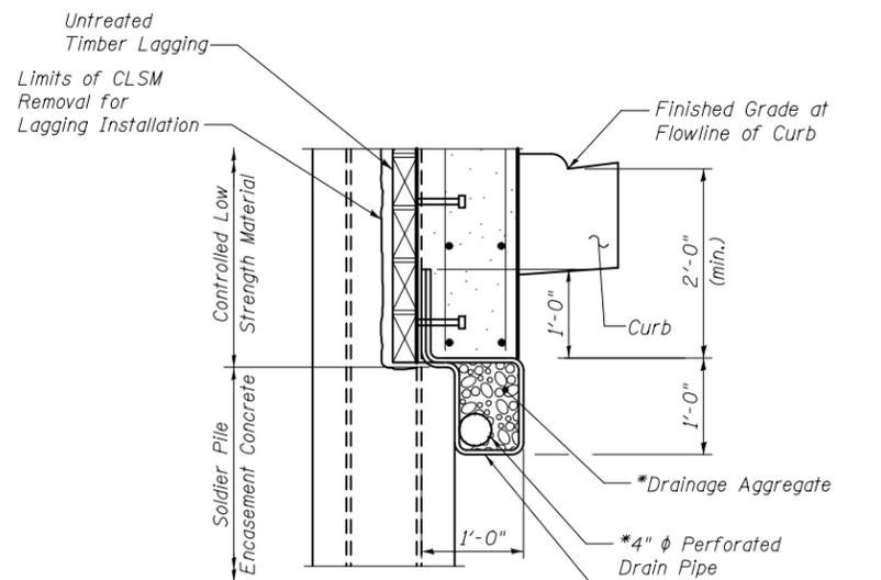
**PIPE UNDERDRAIN DETAIL AT SOLDIER PILES**
