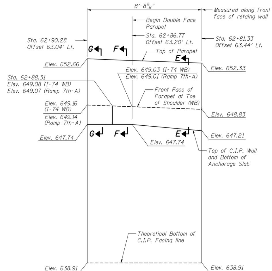
**ELEVATION VIEW OF C.I.P. FACING ALONG I-74 WB**
