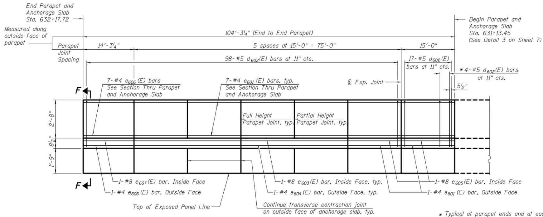
**OUTSIDE ELEVATION OF RAMP 7th-A PARAPET**
