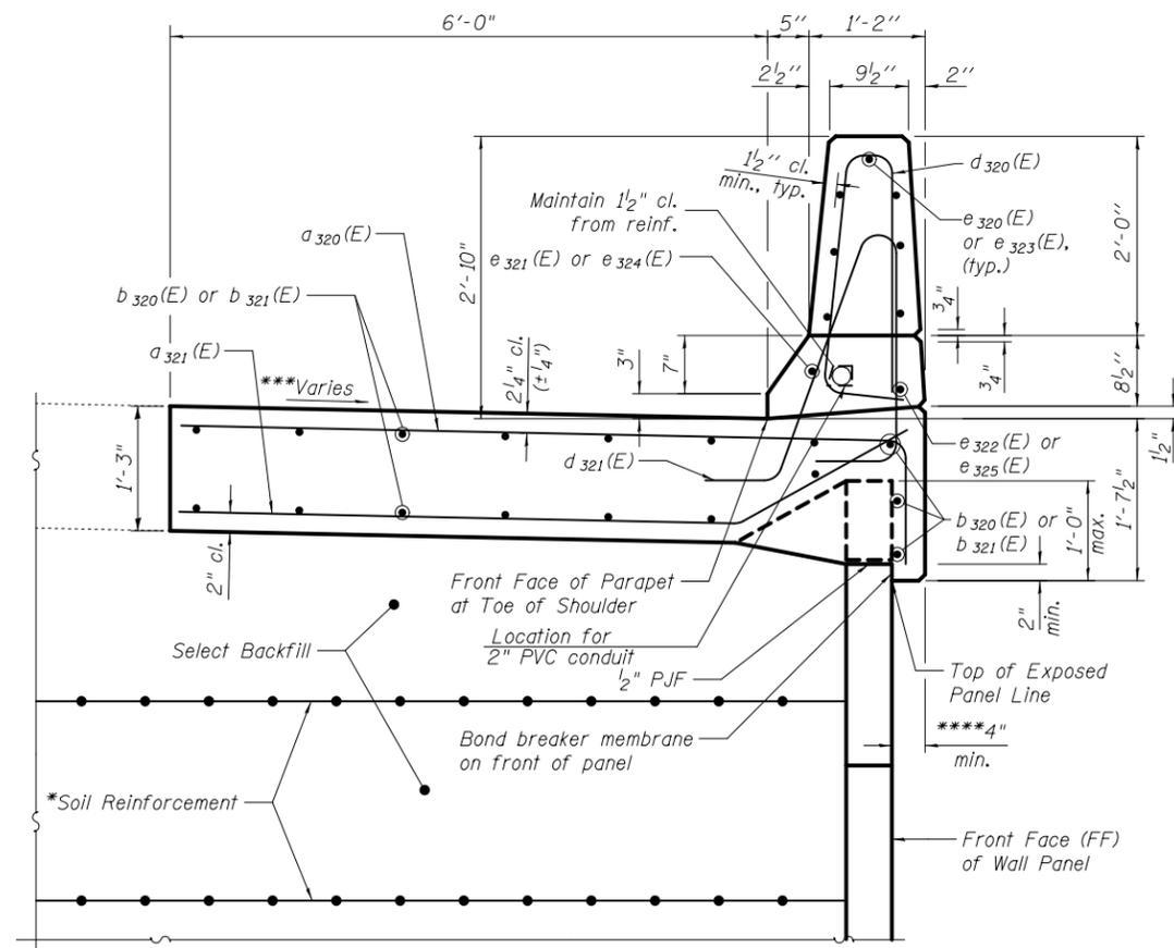
**SECTION THRU PARAPET AND ANCHORAGE SLAB**
