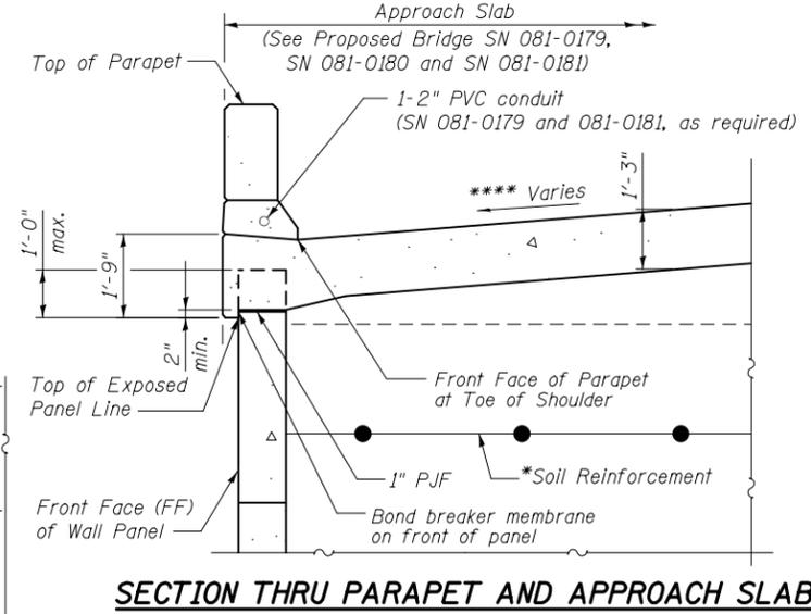
**SECTION THRU PARAPET AND APPROACH SLAB**
