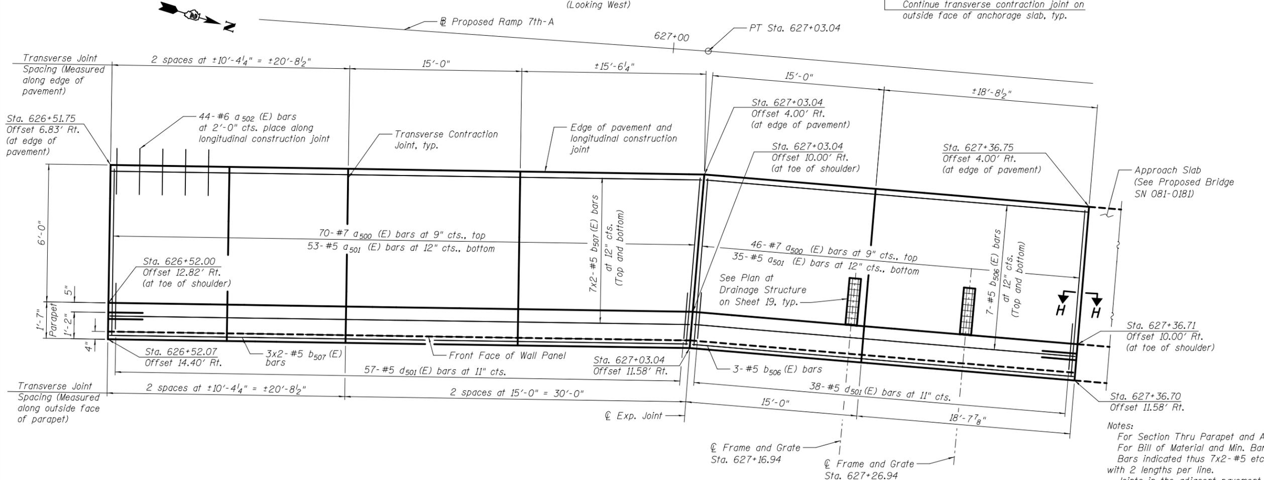
**PLAN - RAMP 7th-A PARAPET AND ANCHORAGE SLAB**
