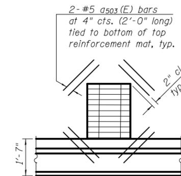
**PLAN AT DRAINAGE STRUCTURE**
