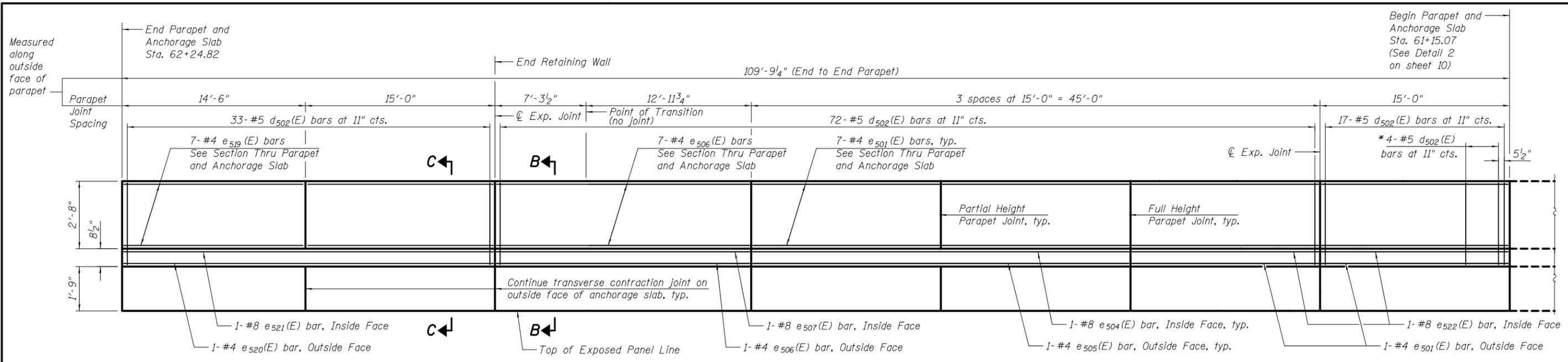
**OUTSIDE ELEVATION OF I-74 EB PARAPET**
