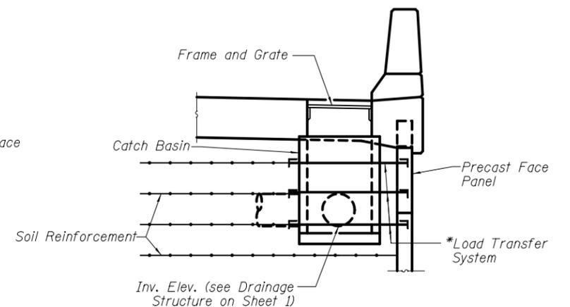
**ANCHORAGE SLAB INLET SECTION**
