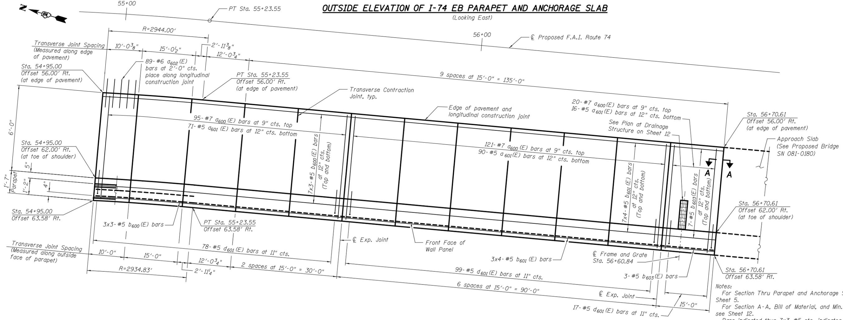
**PLAN - I-74 EB PARAPET AND ANCHORAGE SLAB**
