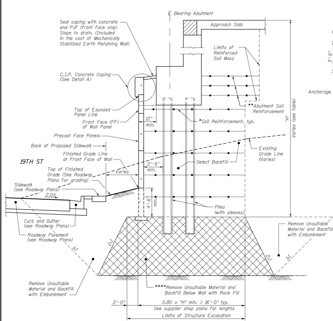
**TYPICAL WALL SECTION THRU ABUTMENT**
