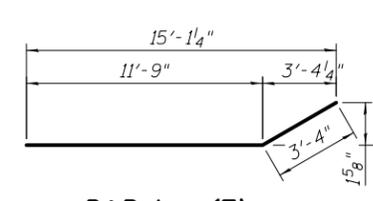
**42" DOUBLE FACE, CONCRETE BARRIER DETAIL**
