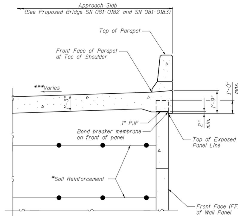
**SECTION THRU PARAPET AND APPROACH SLAB**
