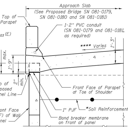
**SECTION THRU PARAPET AND APPROACH SLAB**
