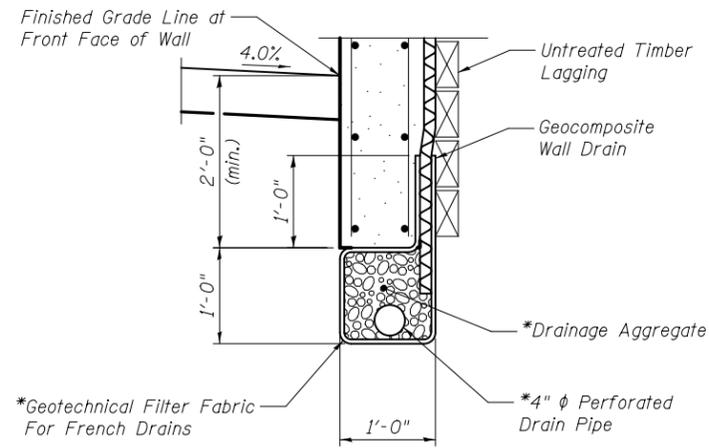
**PIPE UNDERDRAIN DETAILS BETWEEN SOLDIER PILES**
