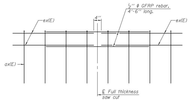
**GFRP REBAR STIFFENING DETAIL**
