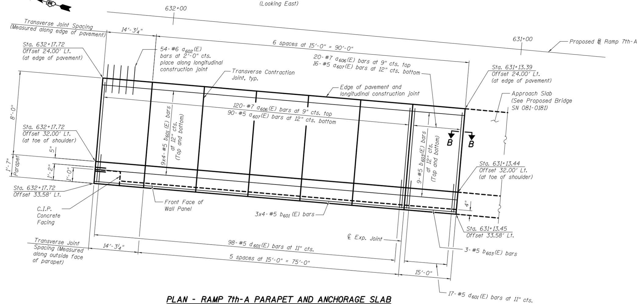
**PLAN - RAMP 7th-A PARAPET AND ANCHORAGE SLAB**
