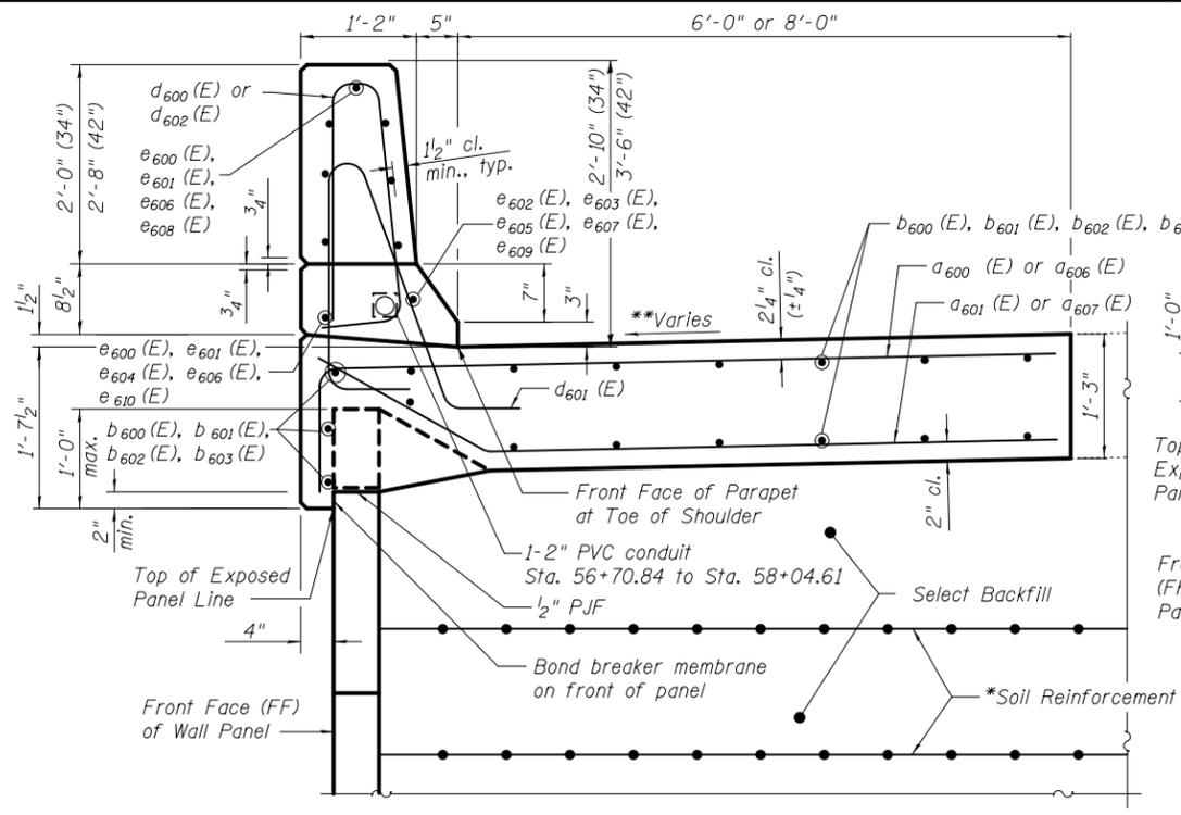
**SECTION THRU PARAPET AND ANCHORAGE SLAB DETAIL**
