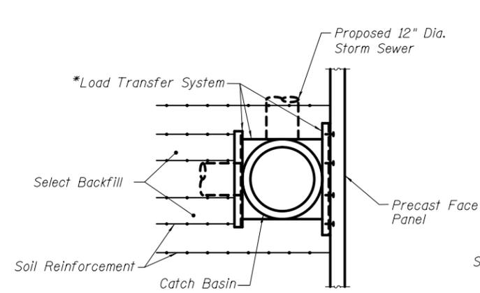
**ANCHORAGE SLAB INLET PLAN**
