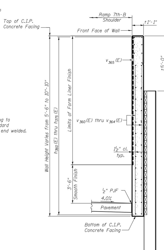
**SECTION THRU CONCRETE FACING**
