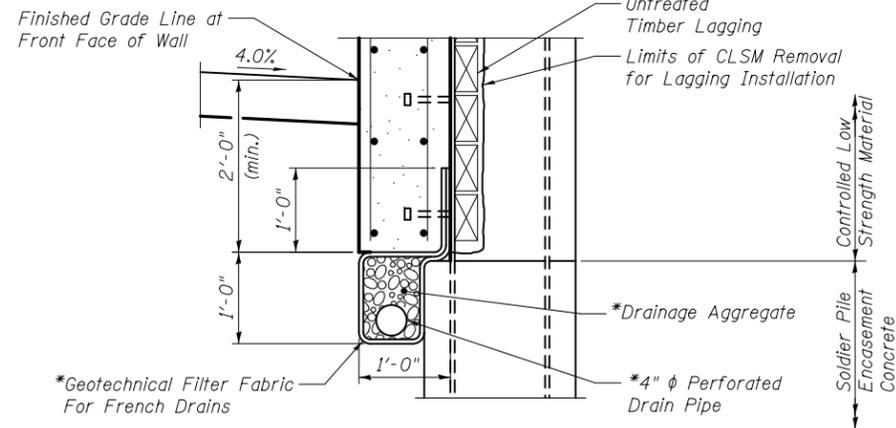
**PIPE UNDERDRAIN DETAILS AT SOLDIER PILES**
