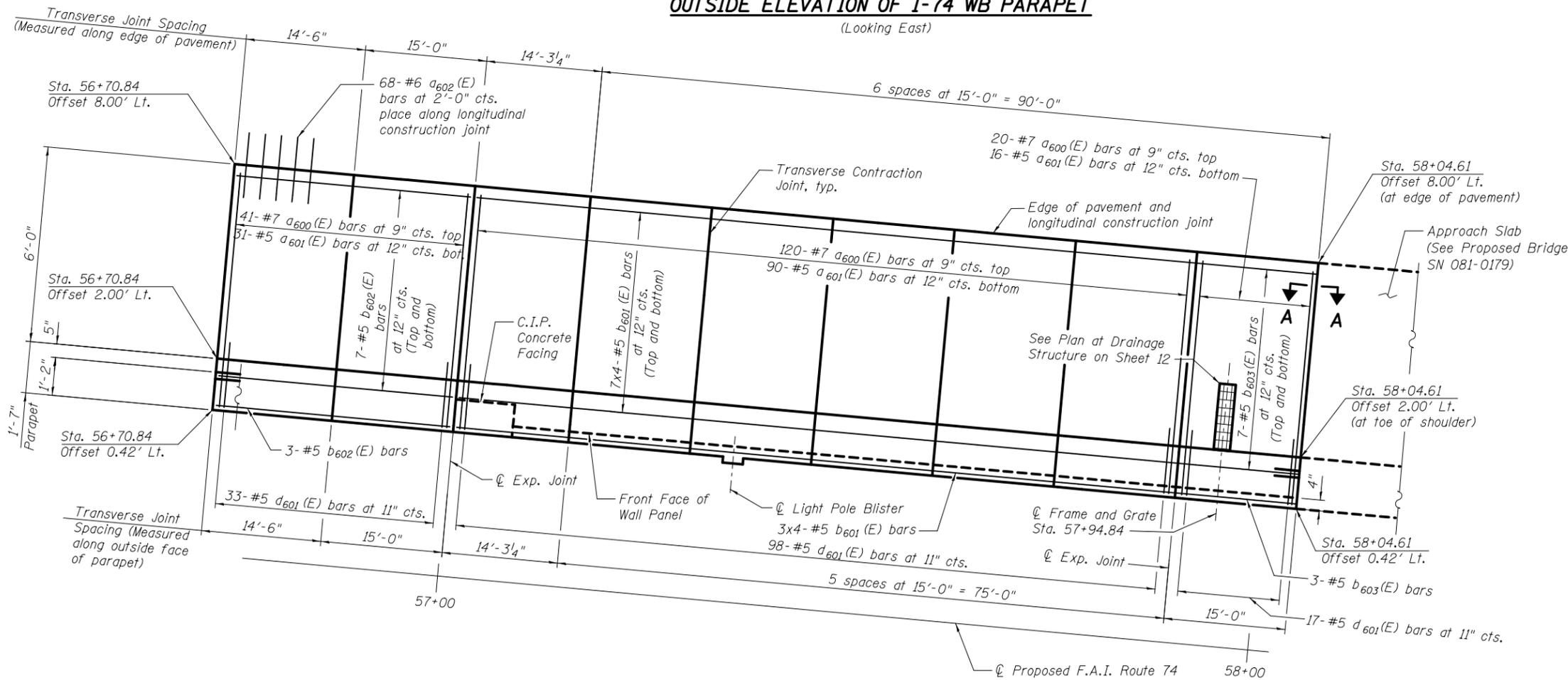
**PLAN - I-74 WB PARAPET AND ANCHORAGE SLAB**
