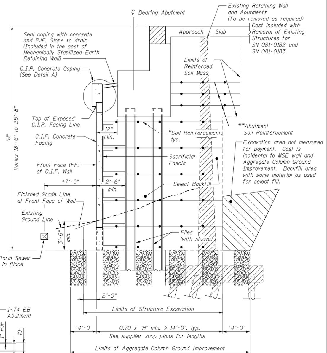
**TYPICAL WALL SECTION THRU ABUTMENT**
