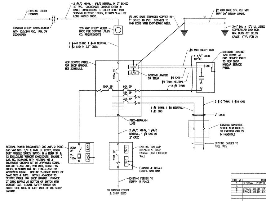
NEW ELECTRICAL ONE-LINE DIAGRAM FOR SHOP HANGAR
