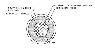
DETAIL A-A € ROADWAY 22'-0" 21'-0" 20'-0" SOUTHBOUND LANES NORTHBOUND LANES \*6 EPOXY COATED REINFORCING STEEL INSERTED INTO CENTER OF SOIL NAIL AND GROUTED. CUTOFF LENGTH-(VARIES) TYPICAL SECTION
