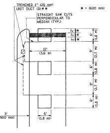
\*\* UNIT DUCT IS TO BE SHOWN ON PLAN SHEETS BUT SHALL NOT BE INCLUDED IN THE PAY ITEMS. NOTE: DUAL LEFT TURNS NOT SHOWN REFER TO PLAN SHEET FOR DETECTOR LOOP REPLACEMENT LEFT TURN LANES WITHOUT MEDIANS
