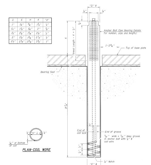
ILLINOIS COIL-LOCK ANCHOR BOLT
