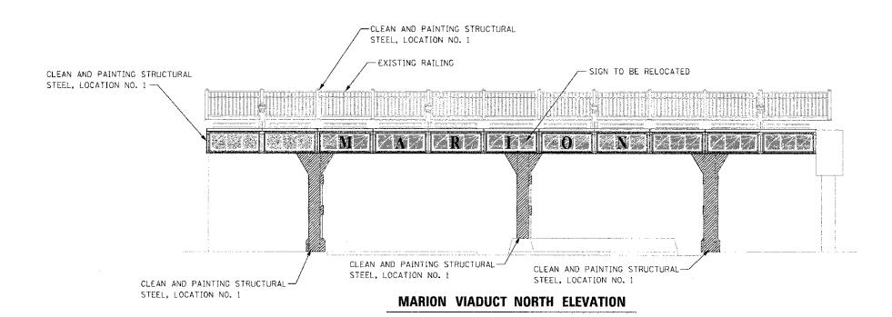
NOTE: ONE ILUMILINE 36 IP OPTIC 30 RGB SHALL BE PROVIDED FOR EACH PANEL OF THE SIGN TO BE RELOCATED. THE FIXTURE, CONDUIT, ELECTRIC CABLE AND ANY OTHER MATERIALS NEEDED TO INSTALL EACH ILUMILINE 36 IP OPTIC 30 RGB SHALL BE INCLUDED IN THE UNIT PRICE OF SIGN TO BE RELOCATED.
