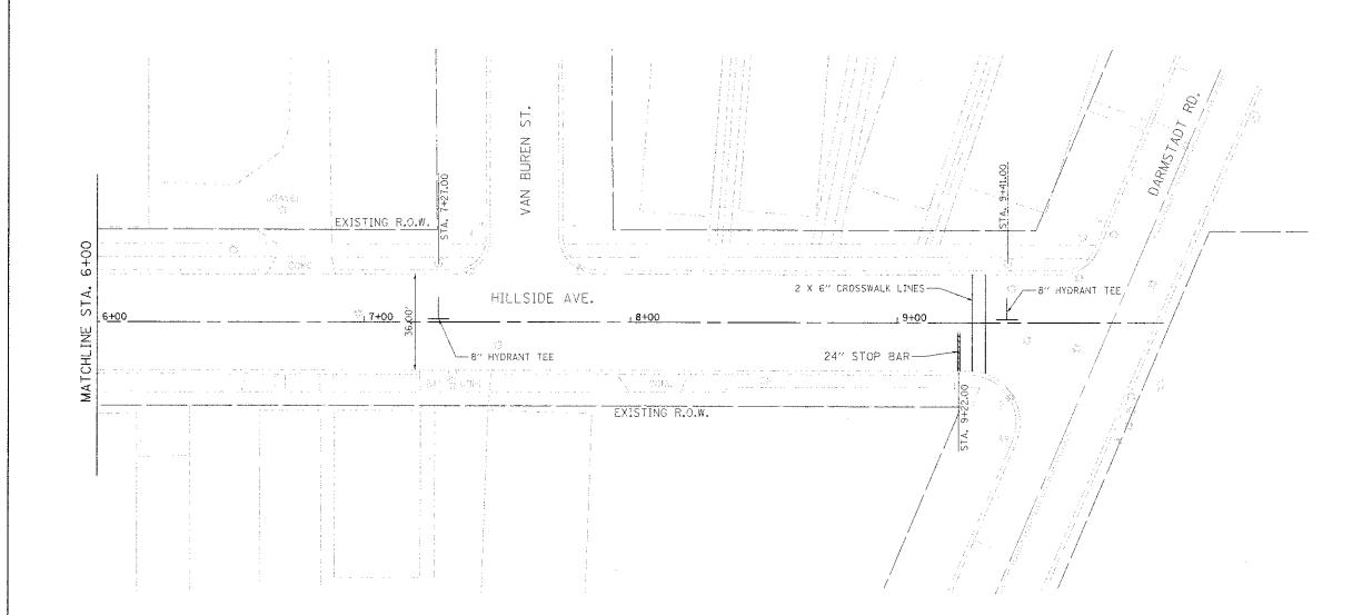
ALL CROSSWALK AND STOP BAR PAVEMENT MARKINGS SHALL IN ACCORDANCE WITH THE LATEST IDOT STANDARDS AND THE MUTCO. STOP BARS NEAR CROSSWALKS SHALL BE LOCATED 4 FEET OFF THE CROSSWALK MARKINGS.
