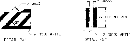
TYPICAL CROSSWALK MARKING
