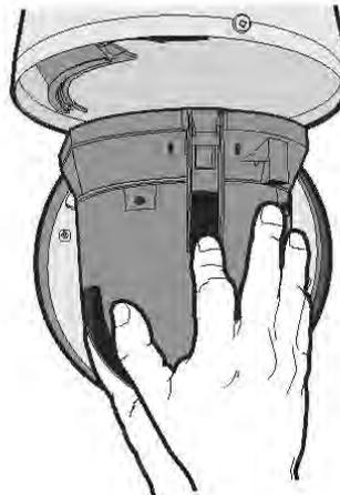
**Figure 2.** Dome Drive Installation
