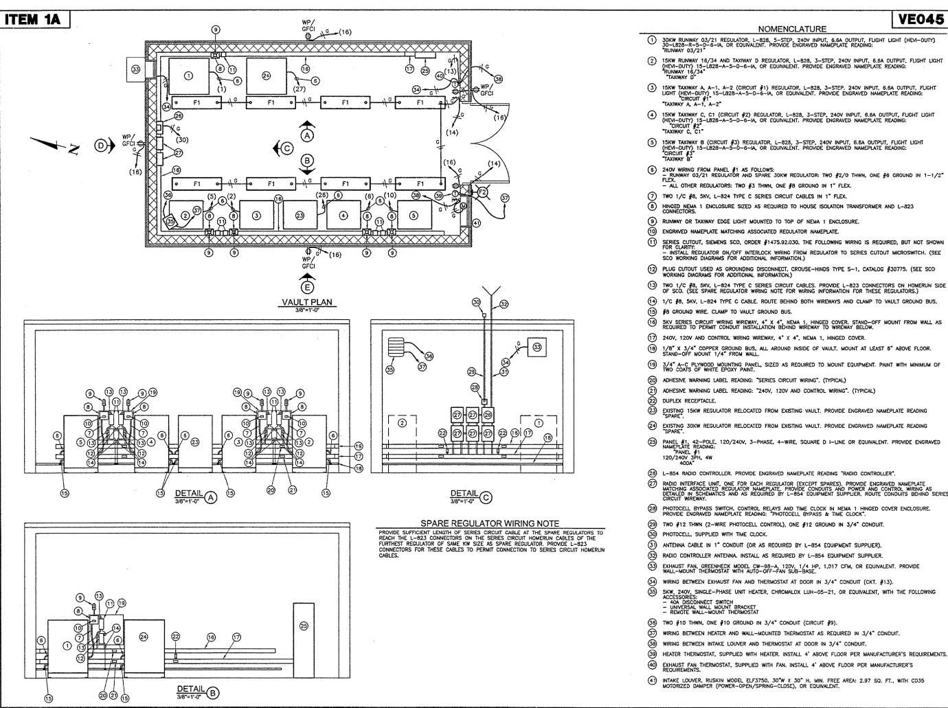
(2) 15KW RUNWAY 16/34 AND TAXIWAY D REGULATOR, L-828, 3-STEP, 240V INPUT, 6.6A OUTPUT, FLIGHT LIGHT (HEVI-DUTY) 15-L828-A-5-D-6-IA, OR EQUIVALENT. PROVIDE ENGRAVED NAMEPLATE READING: "RUNWAY 16/34"
