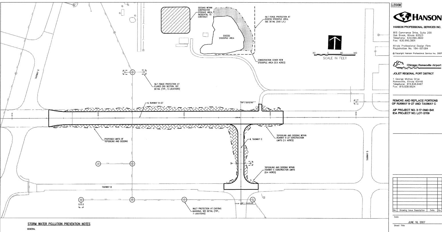
THE CONTRACTOR SHALL IMPLEMENT ALL PROVISIONS OF THE CONTRACT DOCUMENTS TO ASSURE THAT STORM WATER POLLUTION PREVENTION ITEMS ARE CONSTRUCTED AND MAINTAINED IN A TIMELY MANNER. SEDIMENTATION MUST NOT BE TRANSPORTED OFF THE CONSTRUCTION SITE. PERMANENT DRAINAGE FEATURES AND VEGETATIVE MEASURES SHALL BE PROVIDED AS SOON AS POSSIBLE.
