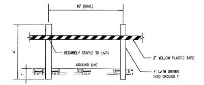
MATERIALS ARE TO BE APPROVED BY ENGINEER PRIOR TO INSTALLATION. COST OF MATERIALS, INSTALLATION, RELOCATION AND MAINTENANCE OLLATHING AND WARNING TAPE IS TO BE INCIDENTAL TO THE CONTRACT.
