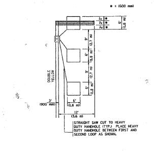
NOTE: QUAL LEFT TURNS NOT SHOWN REFER TO PLAN SHEET FOR DETECTOR LOOP REPLACEMENT
