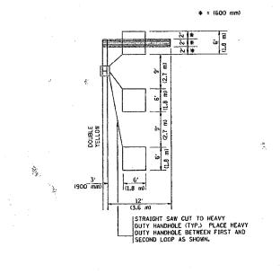
NOTE: DUAL LEFT TURNS NOT SHOWN REFER TO PLAN SHEET FOR DETECTOR LOOP REPLACEMENT
