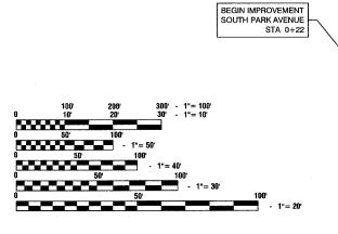
FULL SIZE PLANS HAVE BEEN PREPARED USING STANDARD ENGINEERING SCALES, REDUCED SIZED PLANS WILL NOT CONFORM TO STANDARD SCALES, IN MAKING MEASUREMENTS ON REDUCED PLANS, THE ABOVE SCALES MAY BE USED.
