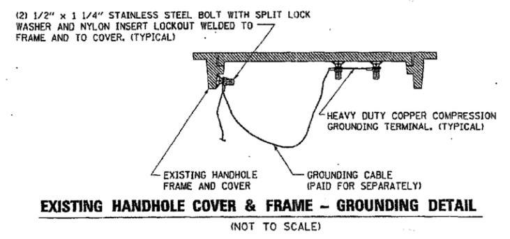
**EXISTING HANDHOLE COVER & FRAME - GROUNDING DETAIL**
