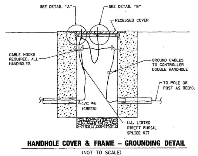
**HANDHOLE COVER & FRAME - GROUNDING DETAIL**
