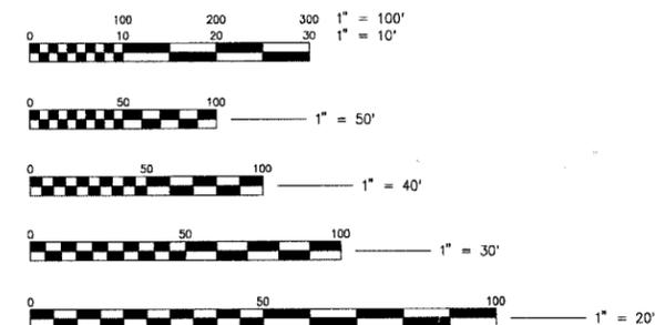
FULL SIZE PLANS HAVE BEEN PREPARED USING STANDARD ENGINEERING SCALES. REDUCED SIZED PLANS WILL NOT CONFORM TO STANDARD SCALES. IN MAKING MEASUREMENTS ON REDUCED SIZE PLANS, THE ABOVE SCALES SHALL BE USED.
