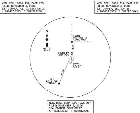
PROPOSED CENTERLINE OF CONSTRUCTION CONTROL TIES
