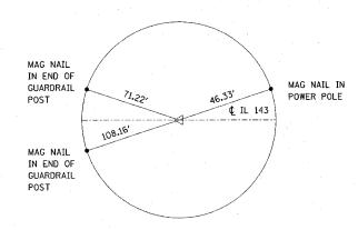
CHISELED "X" ON EAST END MAG NAIL IN OF HEADWALL POWER POLE ¢ IL 143 CHISELED "X" ON CENTER OF HEADWALL
