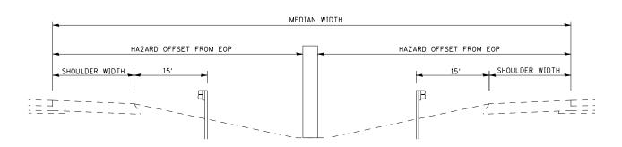
SECTION A-A (TYPICAL CROSS SECTION)
