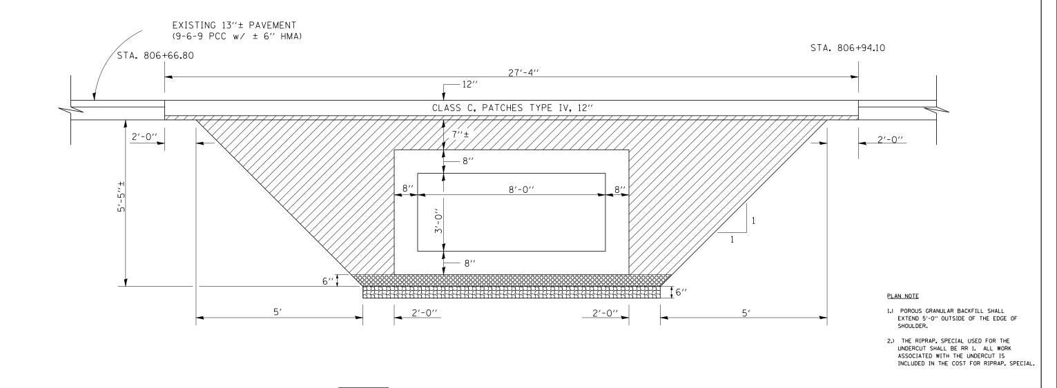
PAY LIMITS OF POROUS GRANULAR BACKFILL-CA 6= 43.0 CU. YD.
