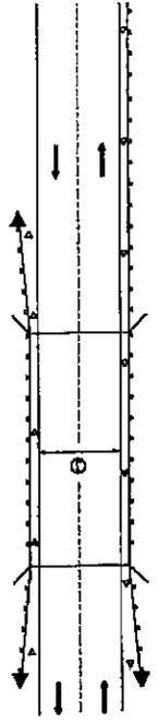
① Bidirectional silver/silver should be used in lieu of monodirectional silver on both sides of two-lane bridges where the bridge pavement approaches the bridge.
