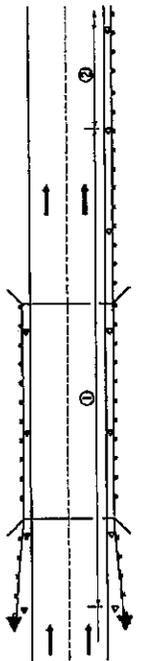
② After 122 m (400 ft.) transition to normal delineator spacing shown in Standard 635001, and continue as required.
