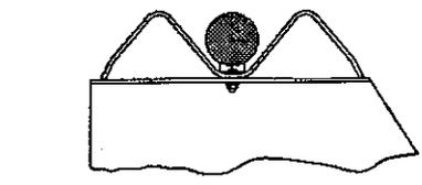
TYPICAL GUARDRAIL MOUNTING WITH REFLECTOR MARKER TYPE A
