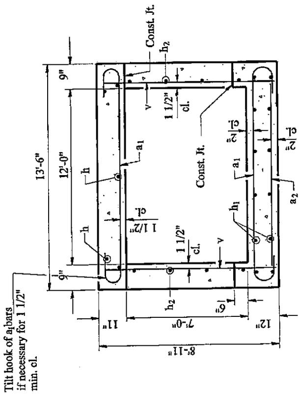
**SECTION THRU BARREL**
