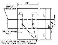
MOUNT DAMPENING PLATE TO END OF EACH TRAFFIC SIGNAL MAST ARM.
