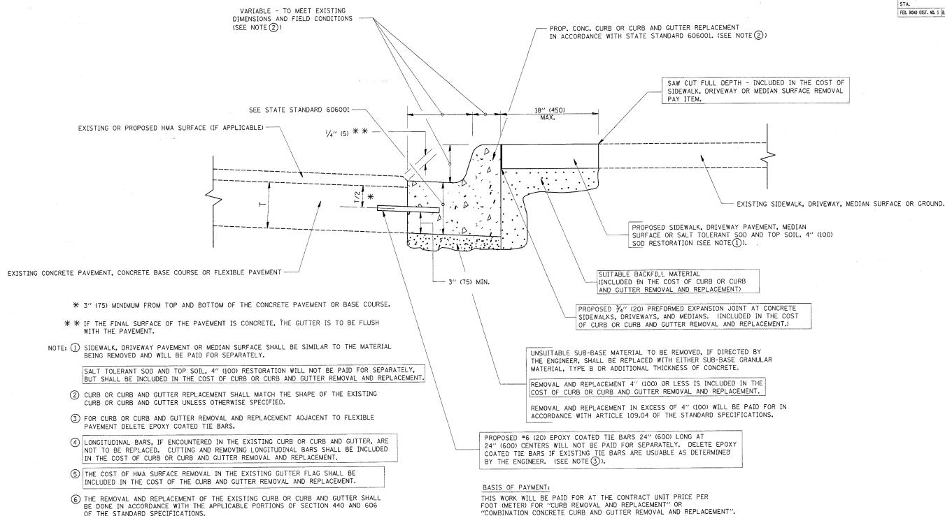
(7) THE LOCATIONS OF REMOVAL AND REPLACEMENT OF EXISTING CURB OR CURB AND GUTTER
