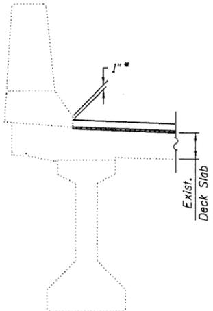
\* Contractor shall increase hydro-scarification thickness or reduce overlay thickness as directed by the Engineer to ensure that this dimension is not less than 0".
