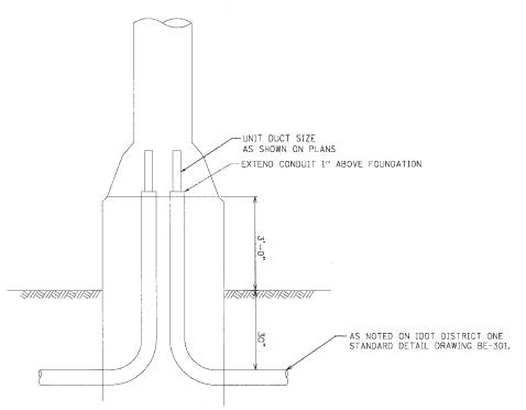
ASSUME THAT REINFORCING STEEL IS ALL INTERCONNECTED VIA TIE WRAPPING OR OTHER SUITABLE MEANS AND CONNECTED TO THE ANCHOR BOLTS.
