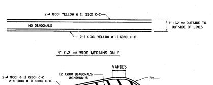
MEDIAN LENGTH FOR MEDIAN LENGTHS WHERE DIAGONAL SPACING CANNOT BE ATTAINED, USE 5 (FIVE) EQUALLY SPACED DIAGONAL LINES.
