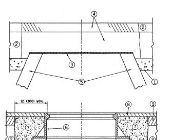
BRICK, MORTAR, OR CONC. ADJUSTING RINGS
