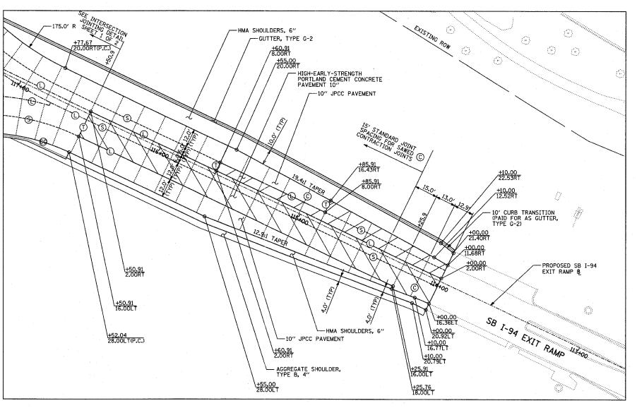
CONSTRUCTION JOINT WITH NO. 6 DEFORMED TIE BAR (EPOXY COATED), 24" LONG @ 24" C-C, DRILL & GROUT IN PLACE (INCLUDED IN THE COST OF CURB & GUTTER OR MEDIAN) SAWED LONGITUDINAL JOINT WITH NO. 6 DEFORMED TIE BAR (EPOXY COATED), 30" LONG & 30" C-C (INCLUDED IN THE COST OF JPCC PAVEMENT) LONGITUDINAL SHOULDER CONSTRUCTION JOINT WITH NO. 8 DEFORMED TIE BAR (EPOXY COATED), 30" LONG & 24" C-C, DRILL & GROUT
