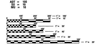
ENGINEERING SCALES. REDUCED SIZED PLANS WILL NOT CONFORM TO STANDARD SCALES. IN MAKING MEASUREMENTS ON REDUCED PLANS, THE ABOVE SCALES MAY BE USED.
