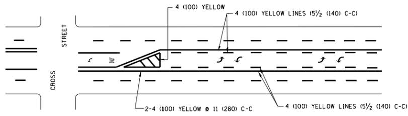
A MINIMUM OF TWO PAIRS OF TURN ARROWS SHALL BE USED, WHITE IN COLOR. ADDITIONAL PAIRS SHALL BE PLACED AT 200' (60 m) TO 300' (90 m) INTERVALS.
