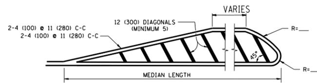
DIAGONAL LINE SPACING: 50' (15 m) C-C (LESS THAN 30MPH (50 km/h))
