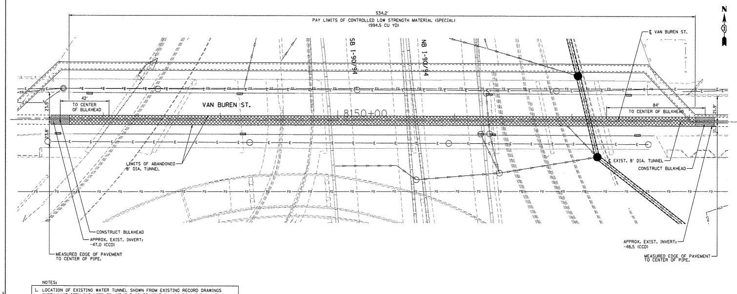
LOCATION OF EXISTING WATER TUNNEL SHOWN FROM EXISTING RECORD DRAWINGS WHICH HAVE BEEN INCLUDED TO AID THE CONTRACTOR IN LOCATING THE EXISTING TUNNEL. THE CONTRACTOR SHALL LOCATE THE EXISTING TUNNEL AS DESCRIBED IN THE SPECIAL PROVISIONS. THIS WORK SHALL BE PAID FOR AS "LOCATE TUNNEL".
