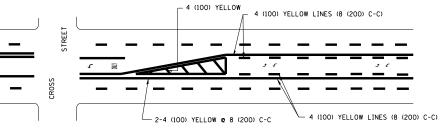
A MINIMUM OF TWO PAIRS OF TURN ARROWS SHALL BE USED, WHITE IN COLOR. ADDITIONAL PAIRS SHALL BE PLACED AT 200' (60 m) TO 300' (90 m) INTERVAL
