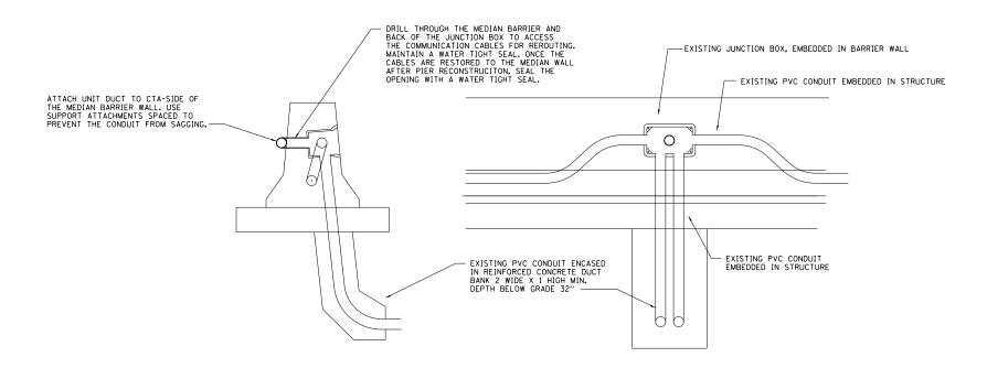
TYPICAL ACCESS TO JUNCTION BOX EMBEDDED IN BARRIER WALL FOR TEMPORARY ITS ROUTING
