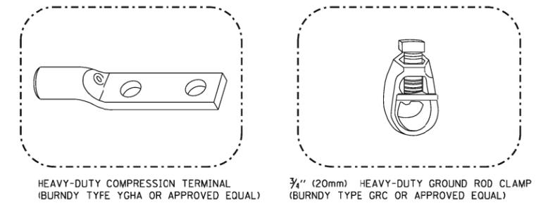
HEAVY-DUTY COMPRESSION TERMINAL (BURNDY TYPE YGHA OR APPROVED EQUAL) 3/4" (20mm) HEAVY-DUTY GROUND ROD CLAMP (BURNDY TYPE GRC OR APPROVED EQUAL)
