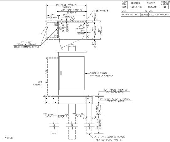
BASED ON CONTROLLER CABINET TYPE IV WITH BASE DIMENSIONS OF 26" x 44" (660mm x 1118mm).
