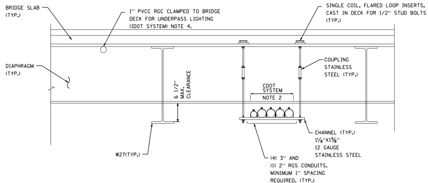
CONDUIT SUPPORT DETAIL UNDER WB 63RD ST. LANES
