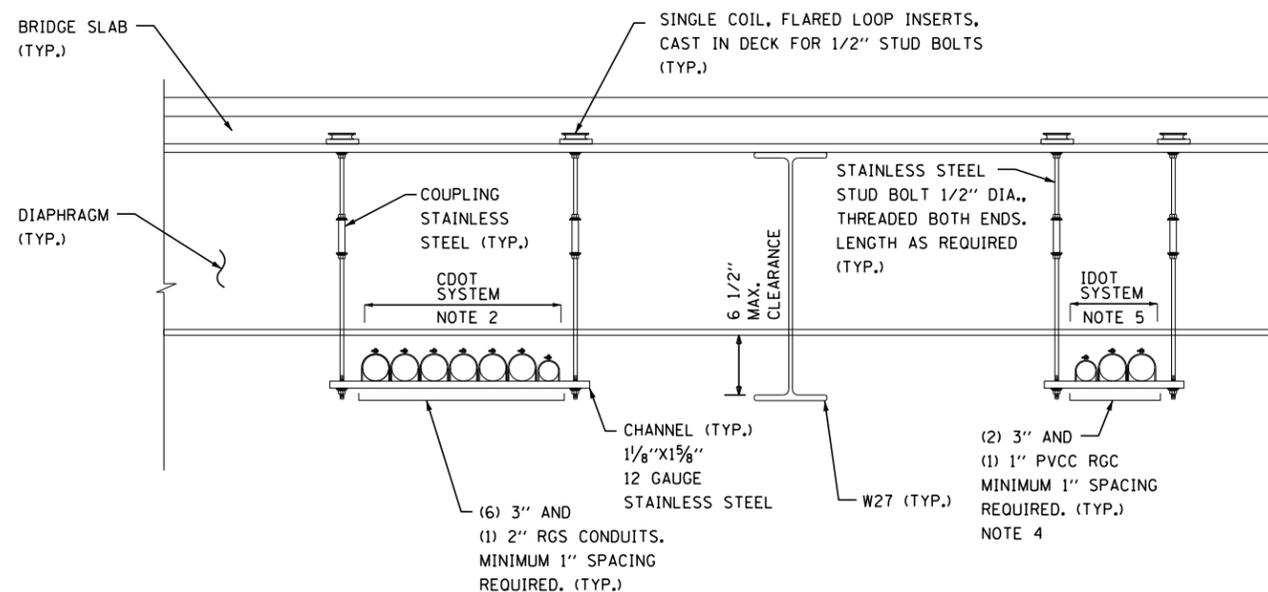
CONDUIT SUPPORT DETAIL UNDER EB 63RD ST. LANES
