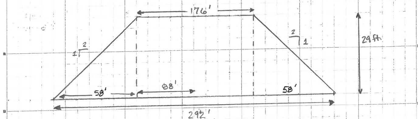
Considering fill will be placed as bridge cone with 2 to 1 sideslopes.
