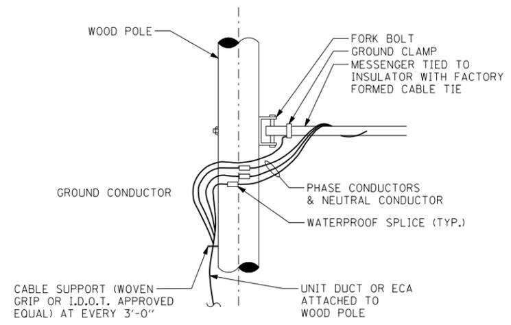
**AERIAL CABLE TO ELECTRIC CABLE ASSEMBLY
