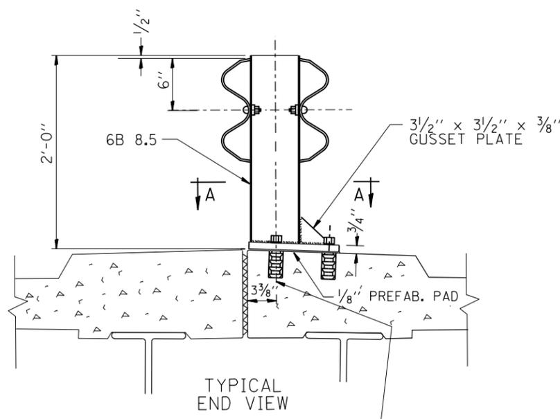
7/8" GALVANIZED ANCHOR BOLTS AND SELF DRILLING EXPANSION SHELLS OR MULTI UNIT TYPE ANCHORS
