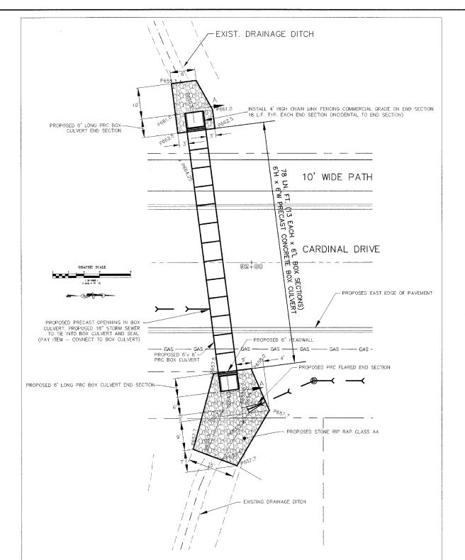
BOX CULVERT (STRUCTURE #4) DETAIL
