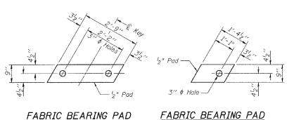
FABRIC BEARING PAD (Exterior and Stage Constr. Line)
