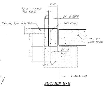
Epoxy grout v(E) bars in drilled holes according to Section 584 of the Standard Specifications, Cost included with Concrete Structures.
